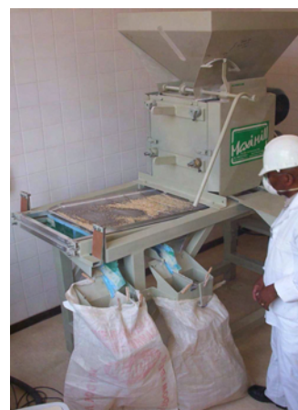
Figure 2. Two roll roller mill used to produce roller milled meal samples.
